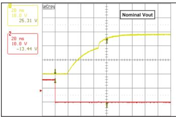
Common Figure 1: Typical startup waveform with 1% load. Input voltage preapplied, ON/OFF Pin on Ch 2.
