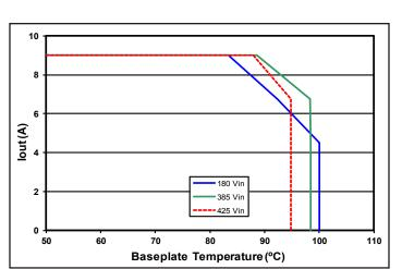
Figure 3:Encased converter max. output power derating vs. base plate temperature.
