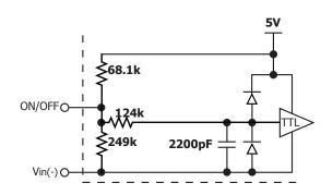
Figure B: Internal ON/OFF pin circuitry
