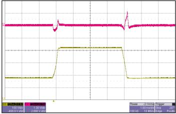
Figure 6: Output voltage response to step-change in input voltage (180V - 425V -270V),(1V/ $\mu$ s) , at 9A load current. Load cap: 15 $\mu$ F tantalum capacitor and 1uF ceramic cap. Ch 1: Vin (100V/div), Ch 2: Vout (1V/div).
